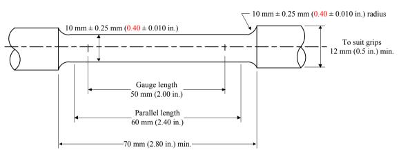
The reduced section may have a gradual taper from the ends toward the center, with the ends not more than Note: 1% larger in diameter than the center (controlling dimension)
