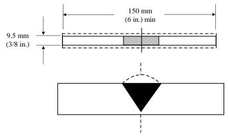
Note Faces of weld to be machined flush with base metal
