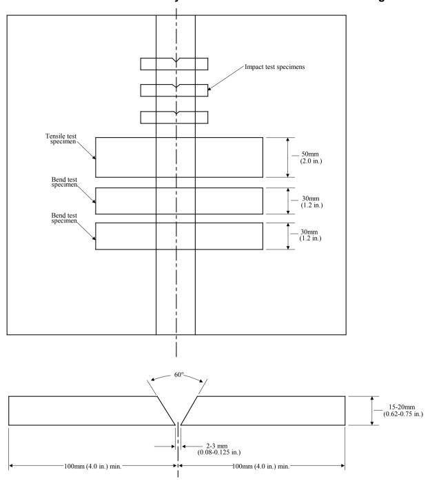
Rules for Materials and Welding Requirements for the Approval of Filler Metals Electrodes for Shielded Metal Arc Welding Appendix 2
