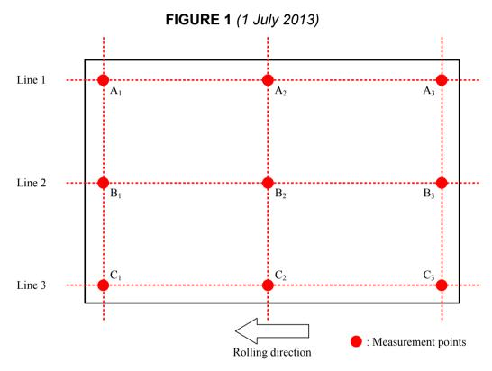
a) Locations of Thickness Measuring Points for the Original Steel Plates
