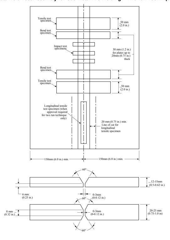
Rules for Materials and Welding Requirements for the Approval of Filler Metals Wire and Wire Gas Combinations for Gas Metal Arc Welding Section
