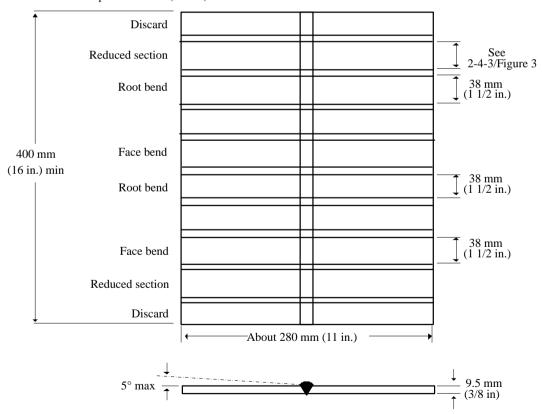
Note: Edge proparation, welding procedure and postweld heat treatment, if any, are to be the same as those for the work represented.
