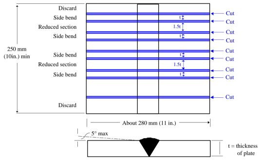
For Plate Up To 19.0 mm (3/4 in.) Thick
