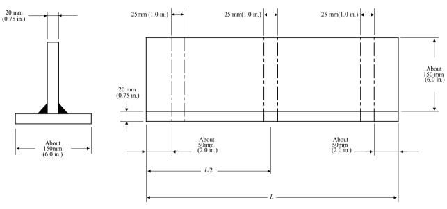
FIGURE 4 **Fillet Weld Hardness Test Locations**
