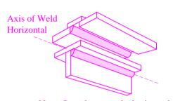
Note: One plate must be horizontal (D) Overhead Position 4F
