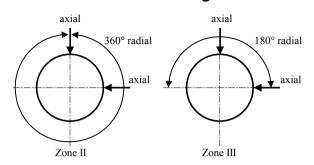
Scanning Direction for Type A and Type B
