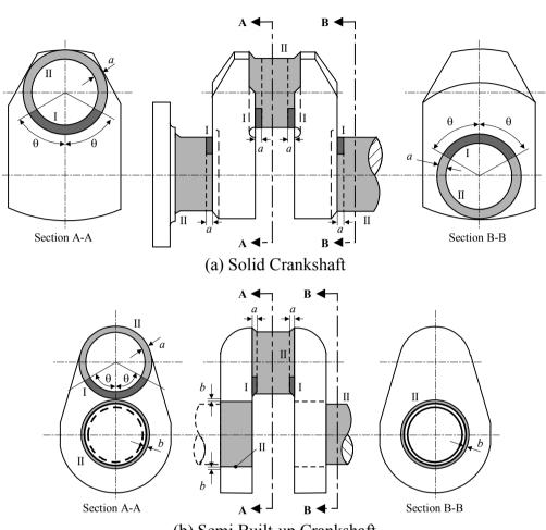
(b) Semi Built-up Crankshaft
