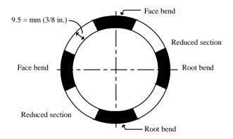
Note: Edge preparation, welding procedure and postweld heat treatment, if any, are to be the same as those for the work represented.
