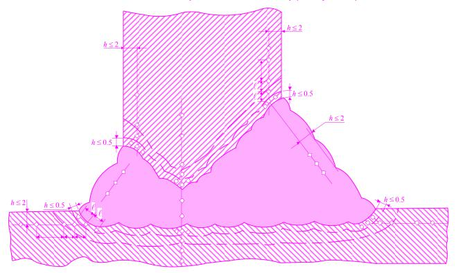
Note: Where the measurement at less than 0.5 mm of heat affected zone from fusion is impractical, the greater distance than 0.5 mm may be accepted.
