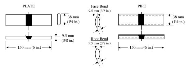
Note: Both faces of weld to be machined flush with base metal.
