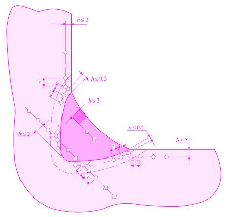
*Note:* Where the measurement at less than 0.5 mm of heat affected zone from fusion is impractical, the greater distance than 0.5 mm may be accepted.
