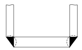
m. Example of corner weld subject to bending stress (not permissible)
