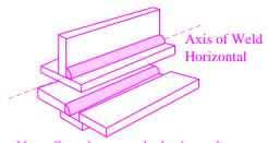
Note: One plate must be horizontal (B) Horizontal Position 2F
