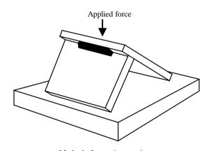
Method of rupturing specimen
