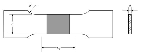
Flat specimen, the weld to be machined (or ground) flush with the surface of the plate, with the following dimensions is to be used:
