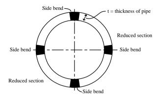
For Pipe Up To 19.0 mm (3/4 in.) Thick
