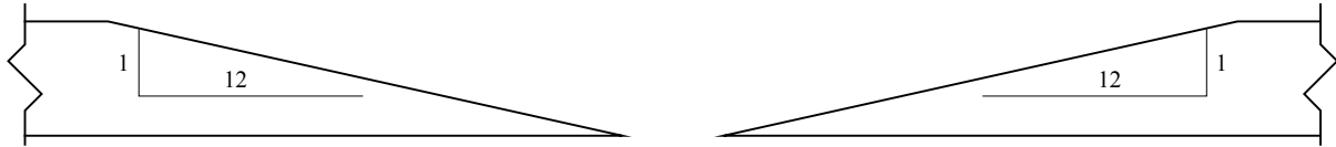
12:1 Tapered Scarf Through Thickness Damage
